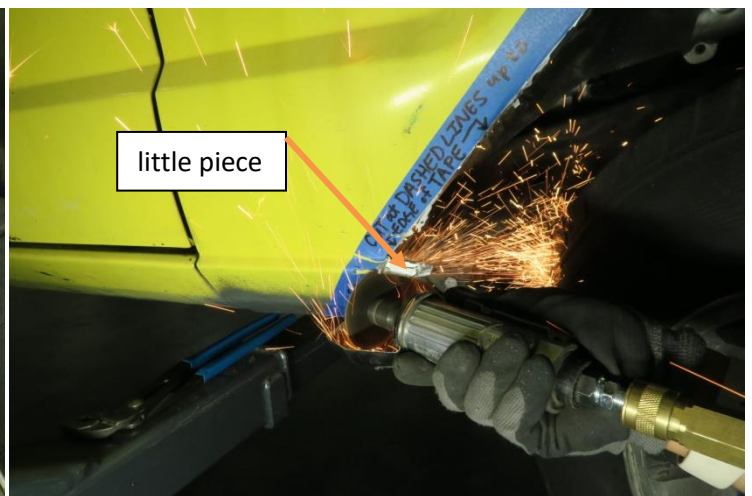
Cut off the little piece remaining from bending the tabs. (Discard)
