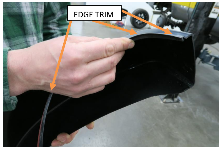
Remove Part from Vehicle and use 1/8" drill bit to create holes at the 4 marks made in the previous step. (Install Edge Trim to the Part during this step.)
