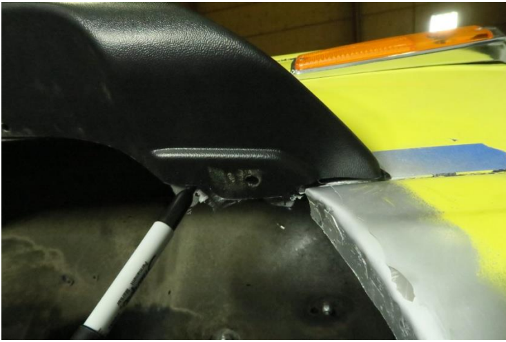
Hold Part in position at the front and mark the metal where it hangs past the edge of the Part.
