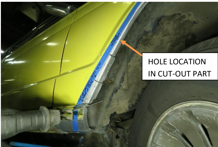
Cut horizontal slices in the rear of the Fender from the wheel well to the edge of tape at the approximate locations in this image. Take care to stay clear of the 'Hole Location' area, and any spot welds.
