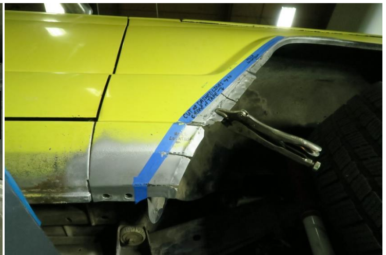
Bend the original Fender Lip flanges out to be parallel with the faces of the Fender, creating tabs.
