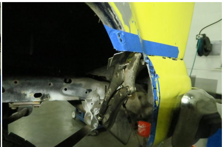
Bend metal under to make horizontal face.
