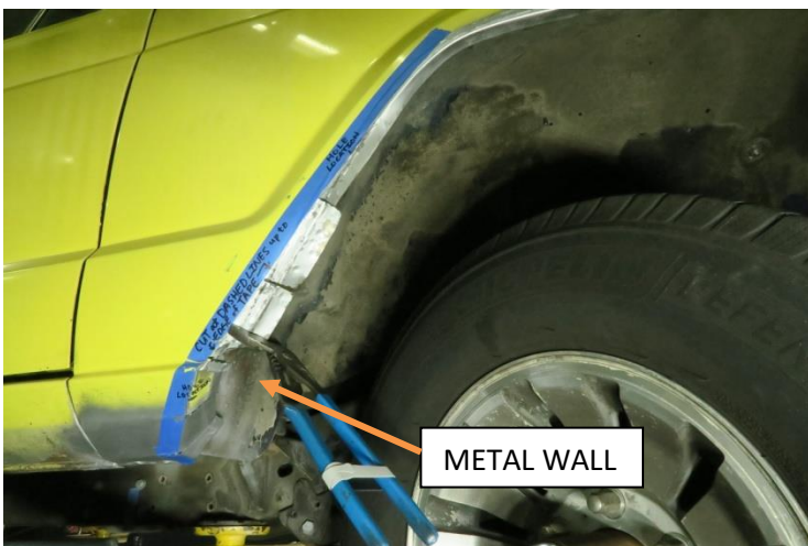
Bend tabs at the tape edge inward to make a new Fender Lip. Hammer tabs flat to lay flush against the metal wall.
