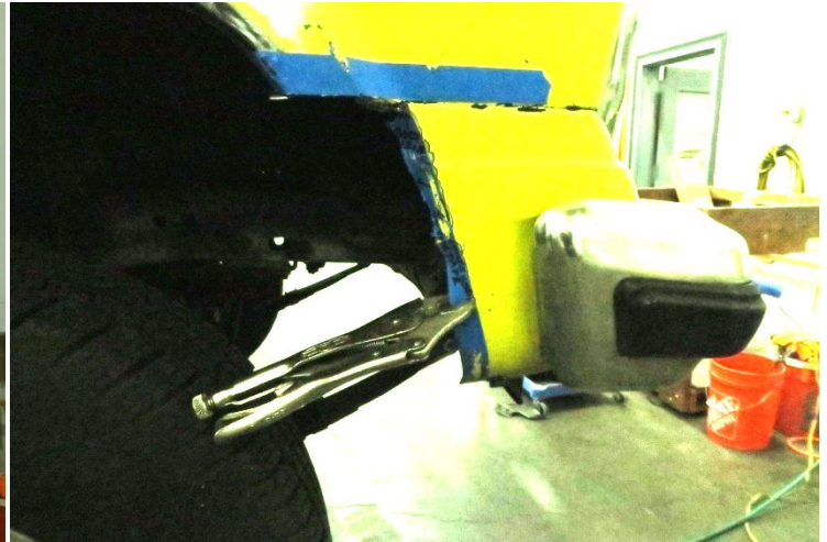
Bend the metal in at the width of the tape. Fold all the way along the tape to make a new Lip.
