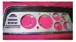
hold the housing to the dash are blocked. You can either use Velcro in this area or not attach them (I prefer the Velcro on the dash & back of the housing). For attachment you have a few options: epoxy, Velcro or 3M double sided emblem tape. Epoxy is messier, but will hold the best. Velcro can come loose in hotter temps. The 3M tape is the easiest and seems to last longer than Velcro, so that's the route I chose.
