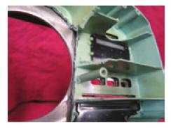
make sure you are on the right track and not removing too much material. Once all the areas are trimmed, you can now install the gauges on the overlay and test-fit to see where the final trimming needs to be.
