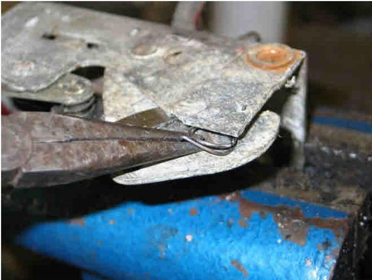
While gently separating the 2 pieces with a flat bladed screwdriver, work this end of the spring into the hole that is in the part of the mechanism that moves (2<sup>nd</sup> hole... see picture below). It may take a couple of tries but it should pop right in.
